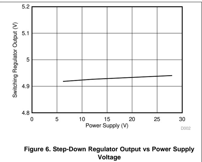
Figure 6. Step-Down Regulator Output vs Power Supply Voltage
