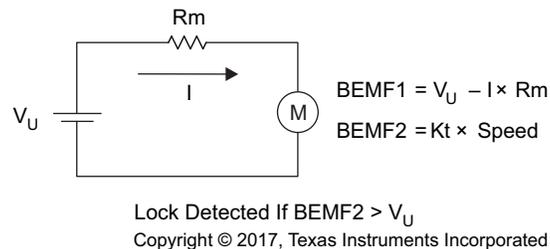
Figure 35. Lock Detection 1
