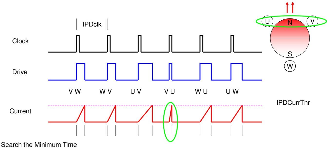
Permanent Magnet ← Saturation Position of the Magnetic Field ← Smallest Inductance ← Minimum Time
