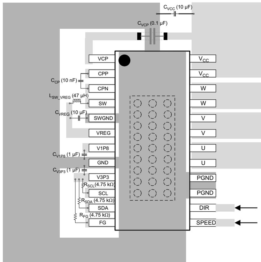
Figure 73. Layout Diagram
