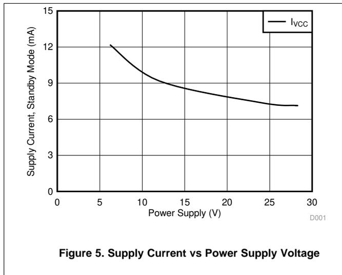
Figure 5. Supply Current vs Power Supply Voltage
