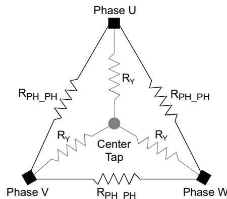
Figure 14. Delta-Connected Motor and the Equivalent Wye Connections
