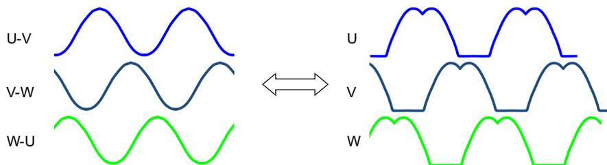
Sinusoidal Voltage From Phase to Phase
