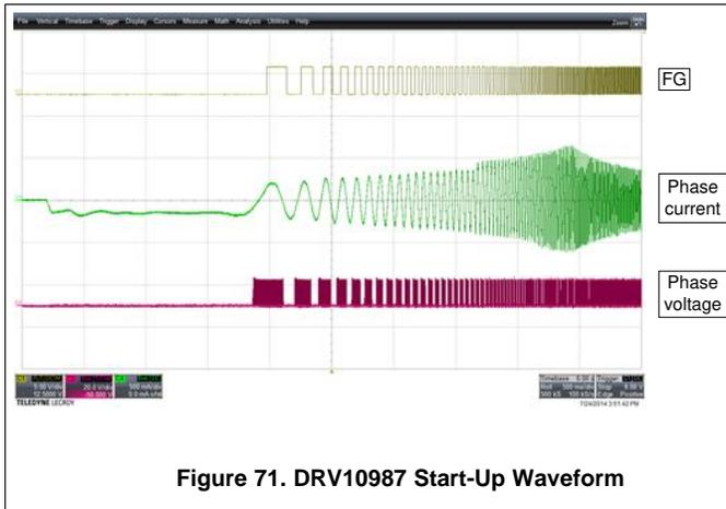
**Figure 71. DRV10987 Start-Up Waveform**
