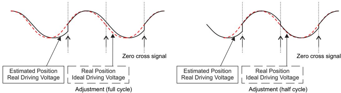
Figure 27. Closed-Loop Control Commutation-Adjustment Mode
