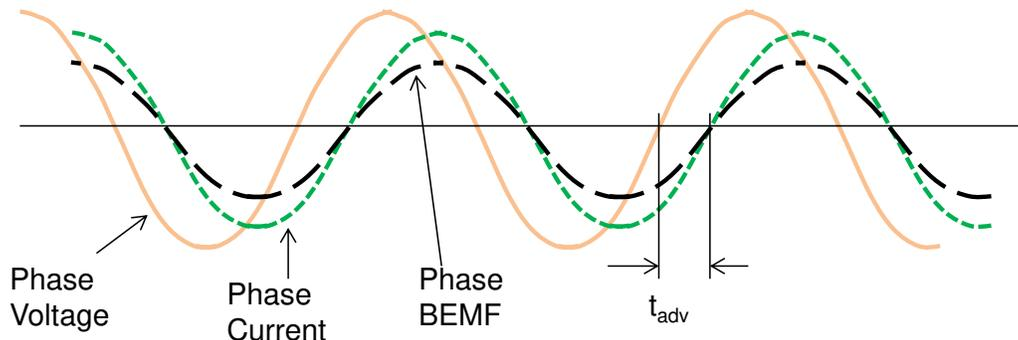
**Figure 31. Advance Time ( $t_{adv}$ ) Definition**
