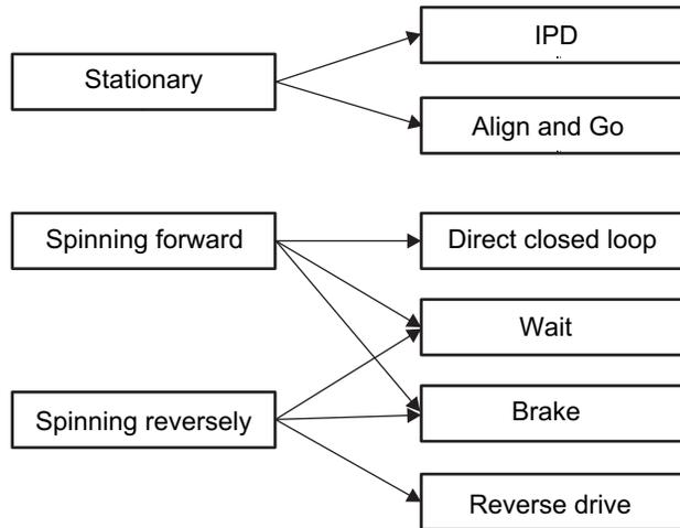
**Figure 16. Start the Motor Under Different Initial Conditions**
